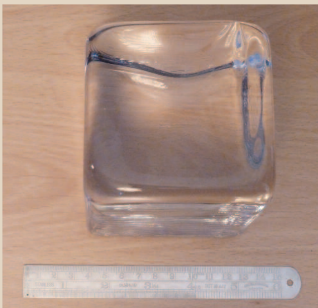
Figure 2 left: A four inch cube of experimental low refractive index glass used to surround the fibres and thus contain the light.
