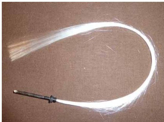
Figure 3. Early glass optical fibres, Image provided by The Museum of Urology, BAUS.
